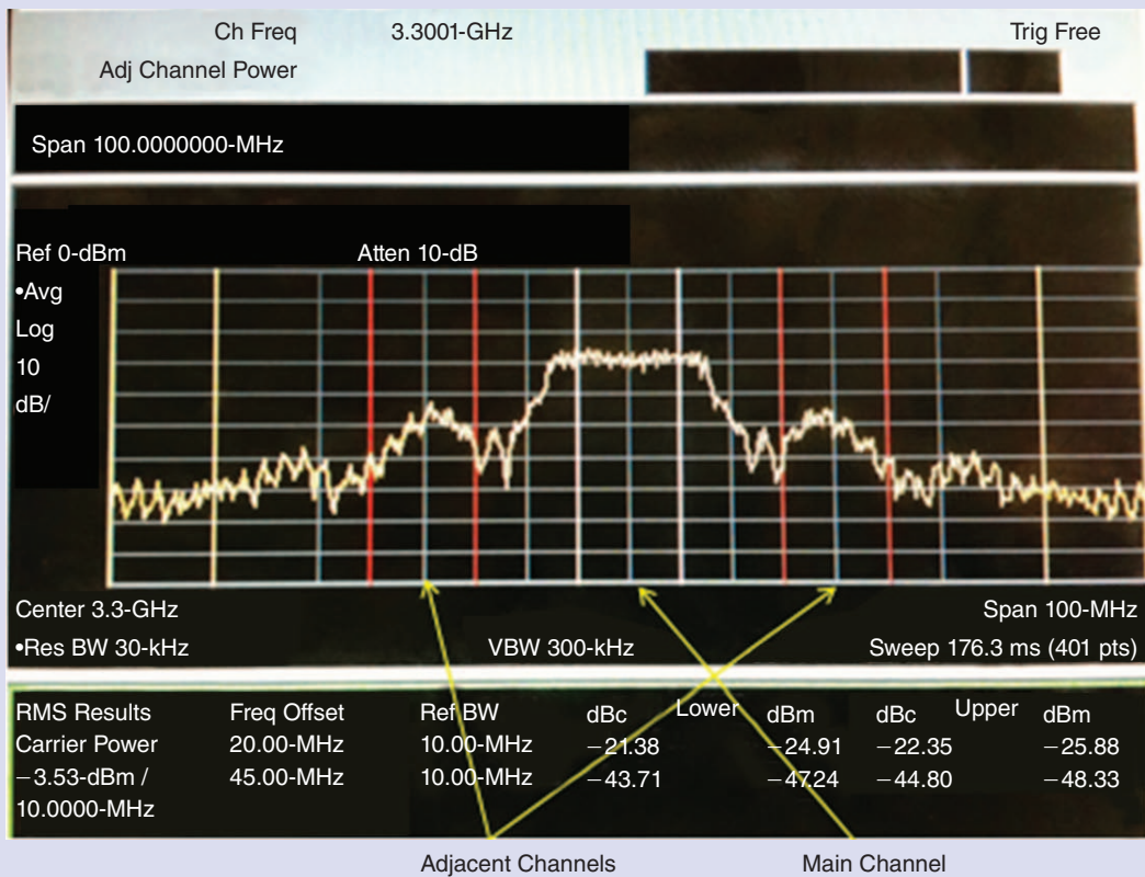
Figure 8. A spectrum analyzer measurement of ACPR. The adjacent channels and main channel are indicated. ACPR is measured by relating the total power in one of the defined adjacent channels to the total measured power in the main channel.
